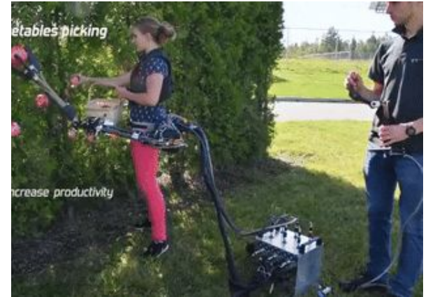
Figure showing a hydraulic wearable arm from Université de Sherbrooke in Canada
